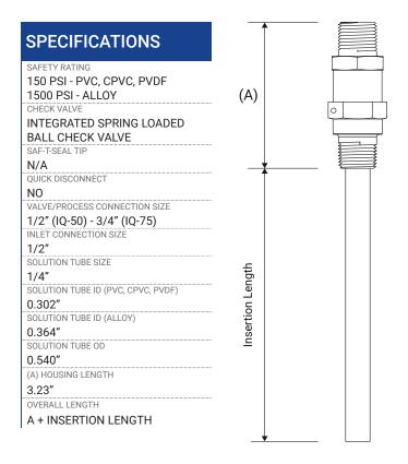
The IQ series non-retractable is well suited to small scale applications or those where the main can easily be depressurized to allow for servicing. The integrated check valve provides convenient isolation from the process pressure. Its size and availability in PVDF, C276, and Alloy20 make it ideal for sulfuric acid applications.
